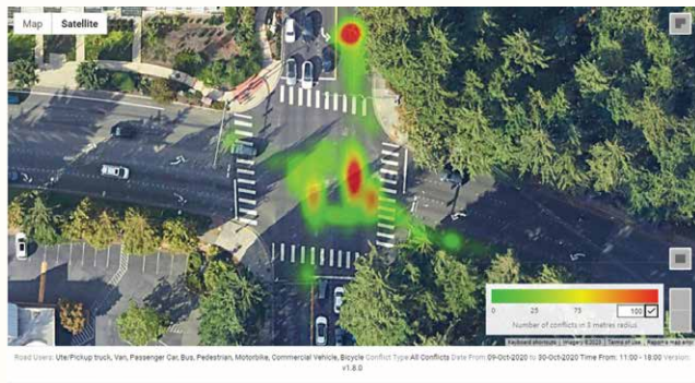
● Conflict heat maps are based on conflict time gaps of less than 1.5 seconds. ● Severity indicates Delta-V (g/s)
