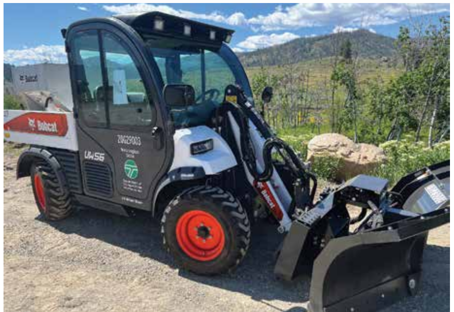
With quick change attachments, the multipurpose UTV owned by WSDOT Eastern Region becomes a snowplow with sander, material loader, mower, and sweeper. Source: WSDOT.
